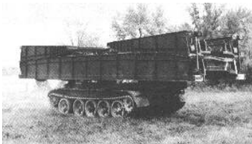
Soviet MTU-20 Tank-Launched Bridge
