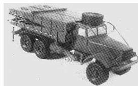
Soviet TMM Truck Mounted Scissors Bridge
